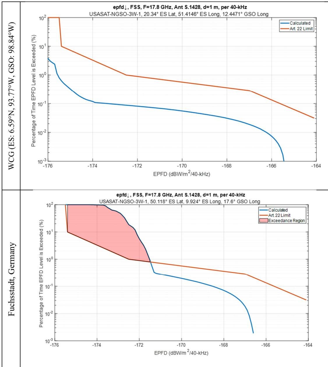
Figure 13 – Comparison of USASAT-NGSO-3W-1 EPFD ↓ in 17.8 – 18.6 GHz Band with 1-m GSO ES for WCG and for Fuchsstadt, Germany (50.118°N, 9.924°E) with GSO Satellite at 17.6°E
