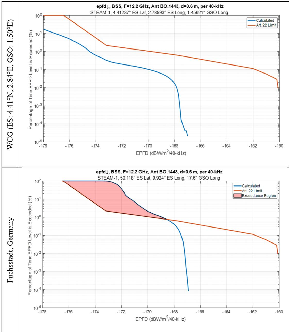
Figure 7 - Comparison of STEAM-1 EPFD ↓ at 12.2 GHz with 0.6 m GSO ES for WCG and for Fuchsstadt, Germany (50.118°N, 9.924°E) with GSO Satellite at 17.6°E
