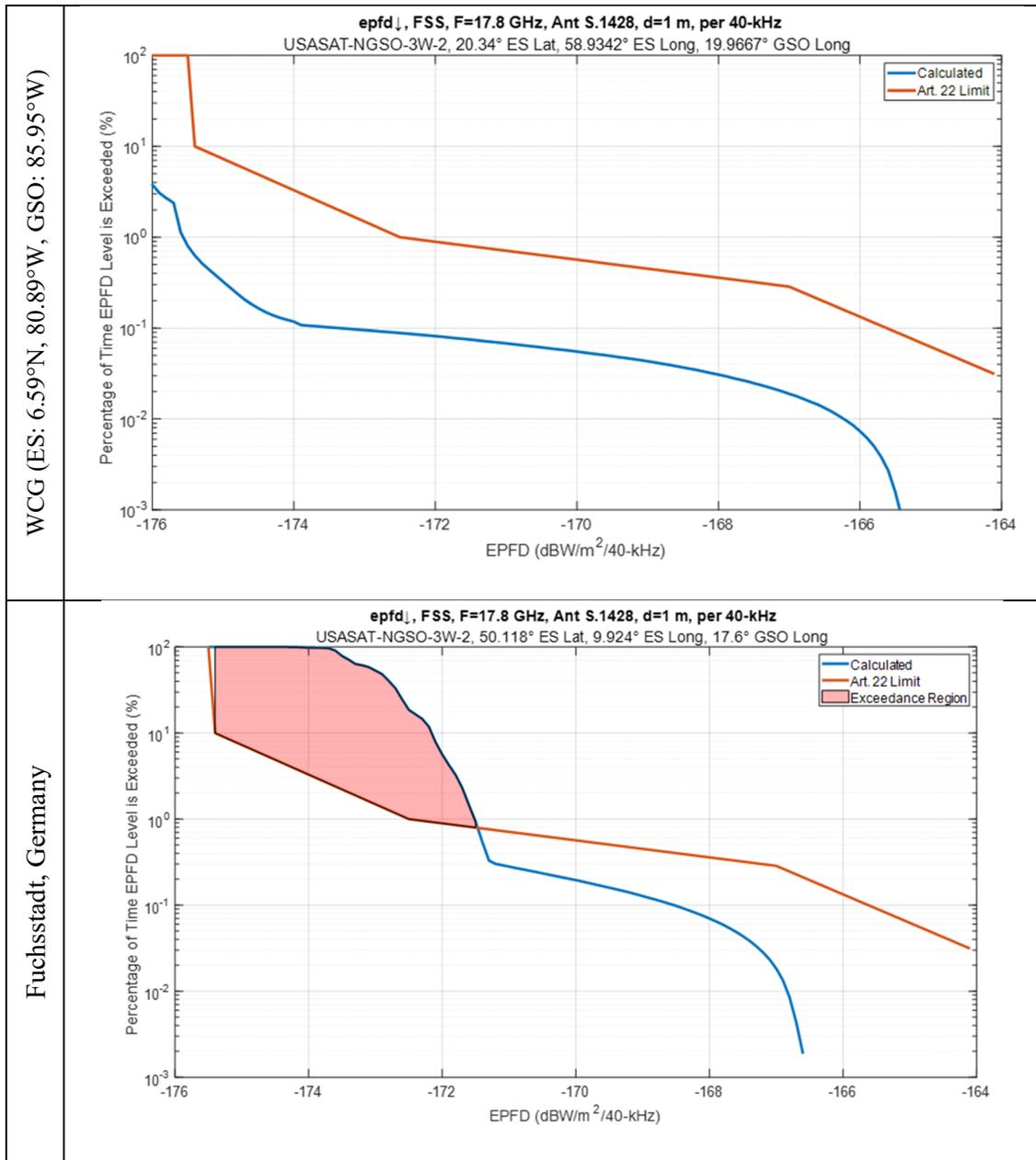
Figure 14 – Comparison of USASAT-NGSO-3W-2 EPFD<sub>↓</sub> in 17.8 – 18.6 GHz Band with 1-m GSO ES for WCG and for Fuchsstadt, Germany (50.118°N, 9.924°E) with GSO Satellite at 17.6°E
