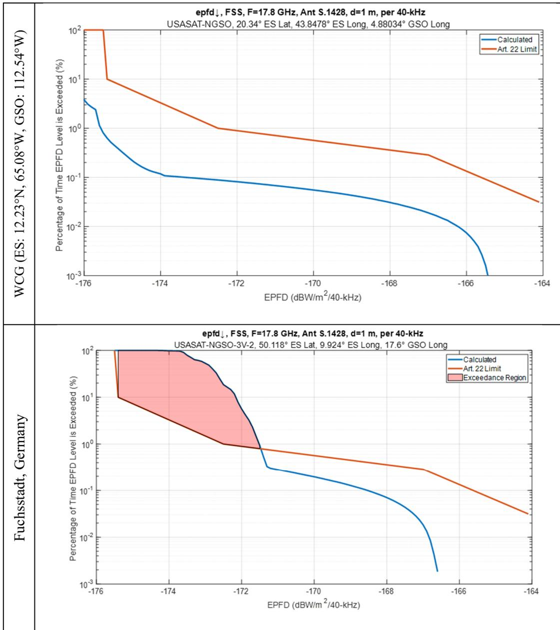
Figure 12 – Comparison of USASAT-NGSO-3V-2 EPFD $\downarrow$  in 17.8 – 18.6 GHz Band with 1-m GSO ES for WCG and for Fuchsstadt, Germany (50.118°N, 9.924°E) with GSO Satellite at 17.6°E
