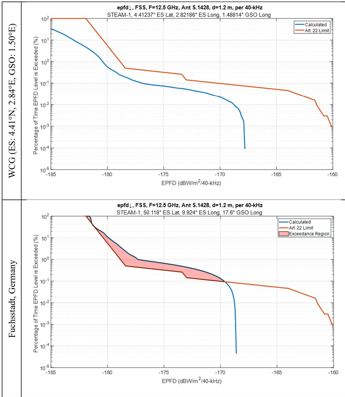
Figure 8 - Comparison of STEAM-1 EPFD $\downarrow$  at 12.5 GHz with 1.2 m GSO ES for WCG and for Fuchsstadt, Germany (50.118°N, 9.924°E) with GSO Satellite at 17.6°E
