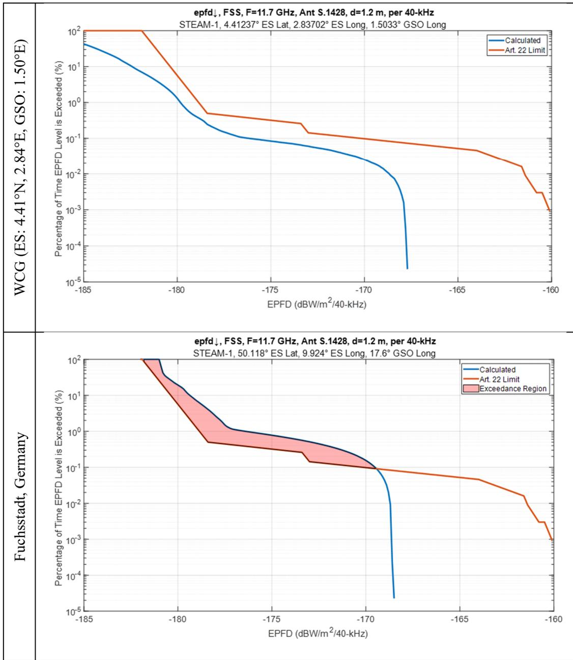
Figure 2 - Comparison of STEAM-1 EPFD<sub>↓</sub> at 11.7 GHz with 1.2 m GSO ES for WCG and for Fuchsstadt, Germany (50.118°N, 9.924°E) with GSO Satellite at 17.6°E
