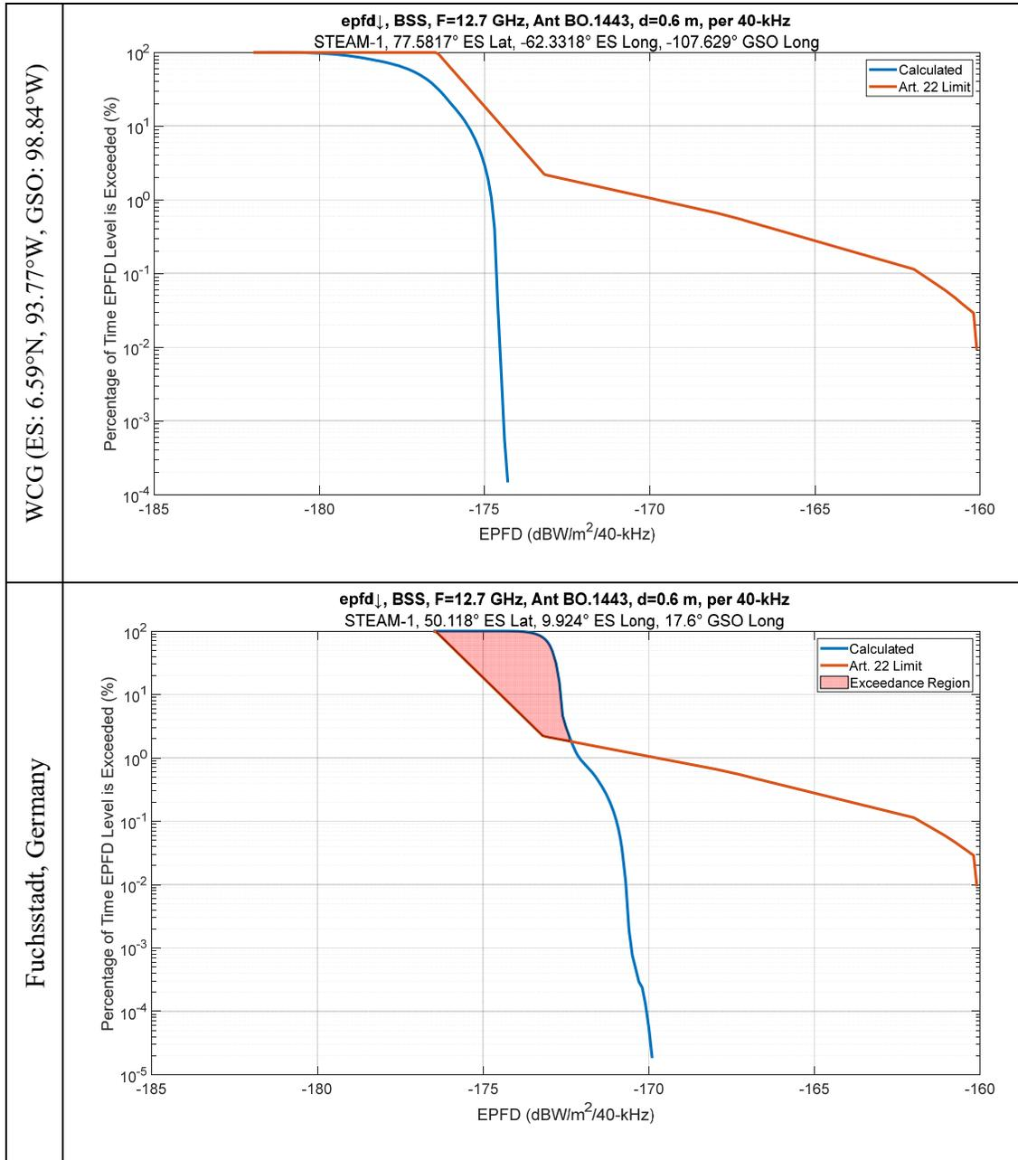
Figure 18 – Comparison of STEAM-1 (ID 121520025) EPFD<sub>↓</sub> at 12.7 GHz with 0.6 m GSO ES for WCG and for Fuchsstadt, Germany (50.118°N, 9.924°E) with GSO Satellite at 17.6°E
