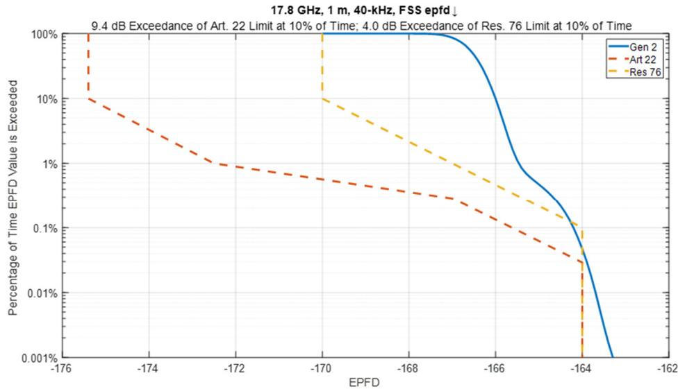
Figure 15 – Combined EPFD ↓ for 29.988 Second Gen2 Starlink Satellites in 17.8 – 18.6 GHz Band with 1-m GSO ES for Fuchsstadt, Germany (50.118°N. 9.924°E) with GSO Satellite at 17.6°E
