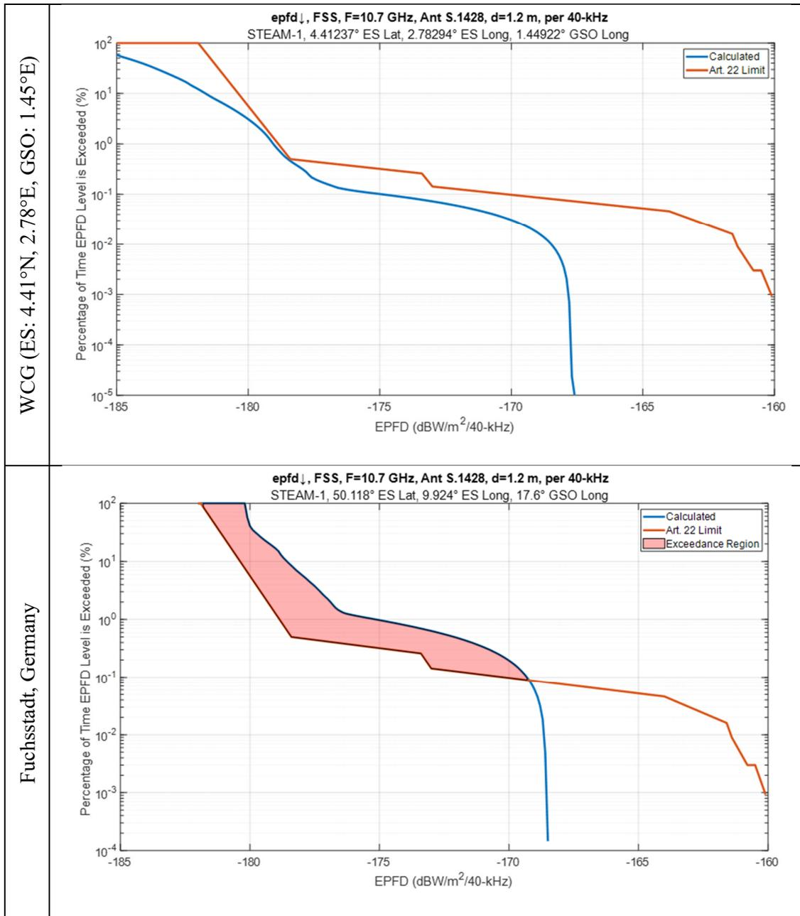
Figure 1 - Comparison of STEAM-1 EPFD ↓ at 10.7 GHz with 1.2 m GSO ES for WCG and for Fuchsstadt, Germany (50.118°N, 9.924°E) with GSO Satellite at 17.6°E
