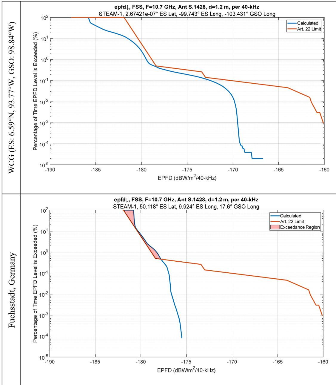
Figure 16 – Comparison of STEAM-1 (ID 121520025) EPFD↓ at 10.7 GHz with 1.2 m GSO ES for WCG and for Fuchsstadt, Germany (50.118°N, 9.924°E) with GSO Satellite at 17.6°E
