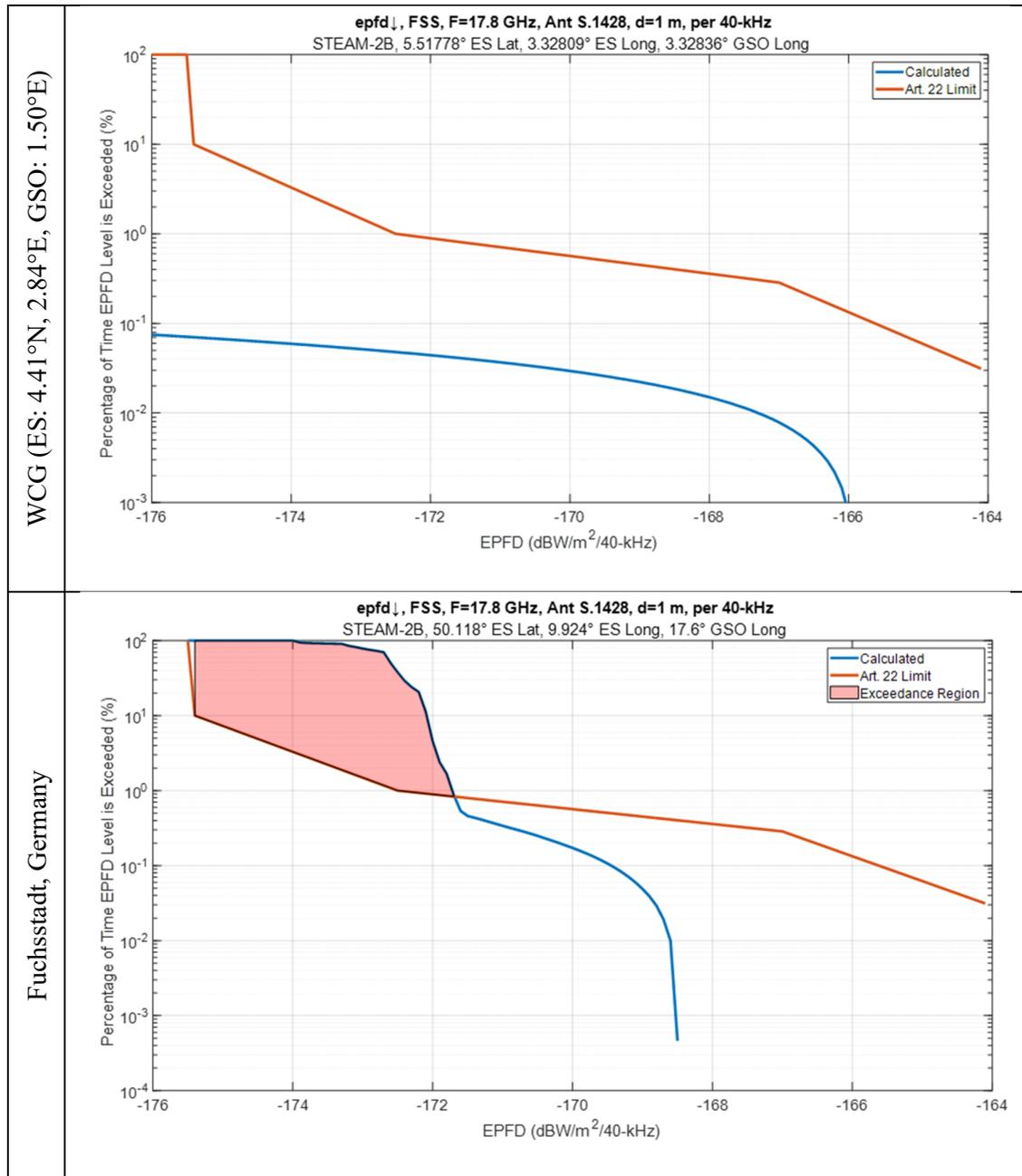
Figure 11 - Comparison of STEAM-2 EPFD ↓ at 17.8 GHz with 1 m GSO ES for WCG and for Fuchsstadt, Germany (50.118°N, 9.924°E) with GSO Satellite at 17.6°E
