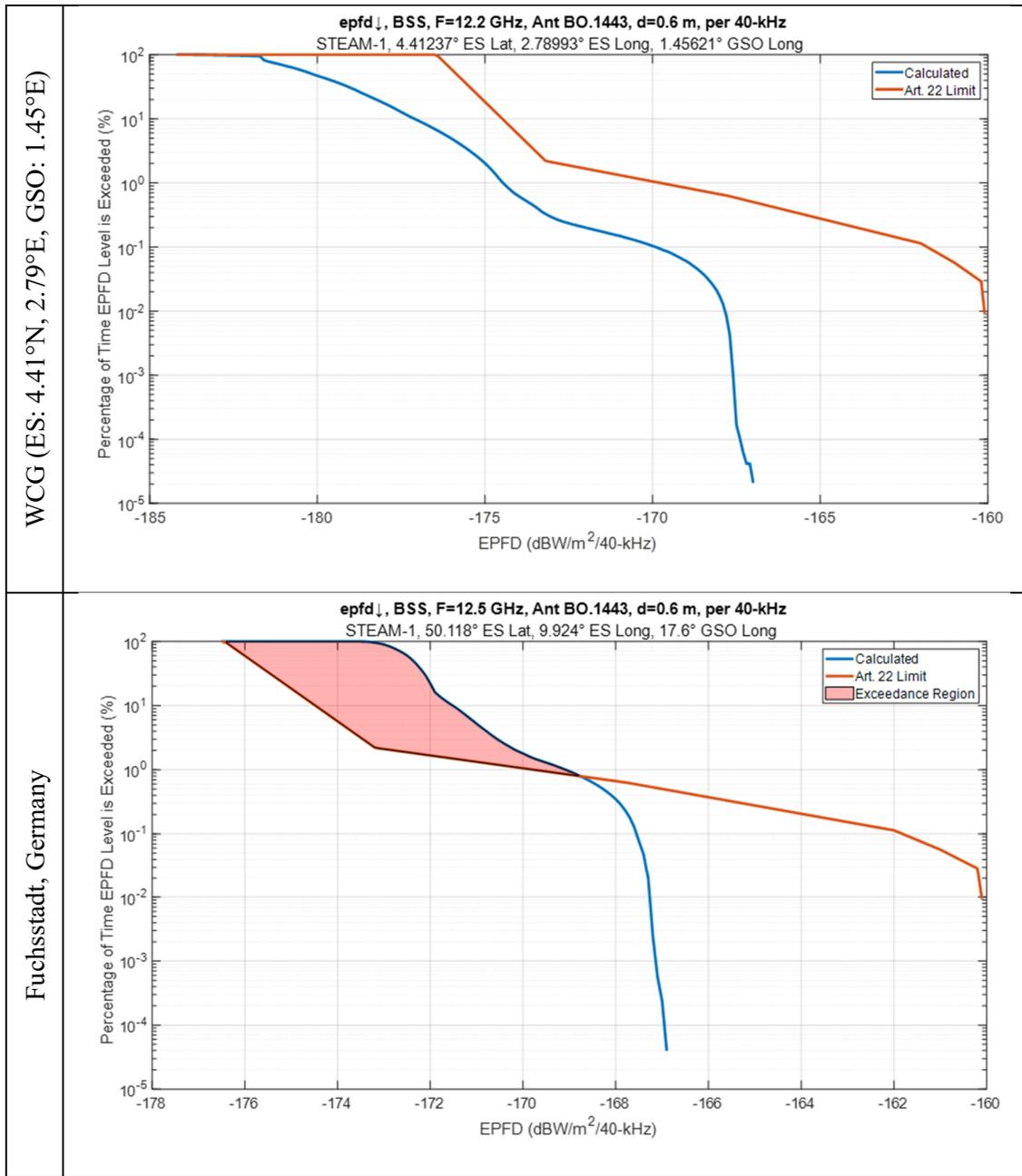
Figure 10 - Comparison of STEAM-1 EPFD ↓ at 12.5 GHz with 0.6 m GSO ES for WCG and for Fuchsstadt, Germany (50.118°N, 9.924°E) with GSO Satellite at 17.6°E
