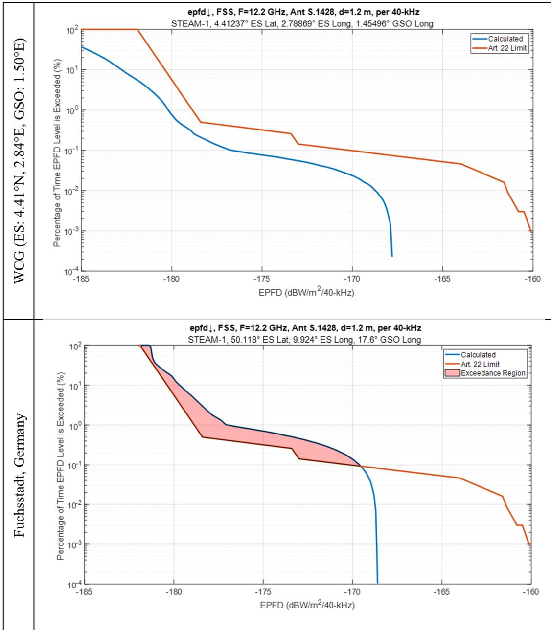
Figure 5 - Comparison of STEAM-1 EPFD↓ at 12.2 GHz with 1.2 m GSO ES for WCG and for Fuchsstadt, Germany (50.118°N, 9.924°E) with GSO Satellite at 17.6°E
