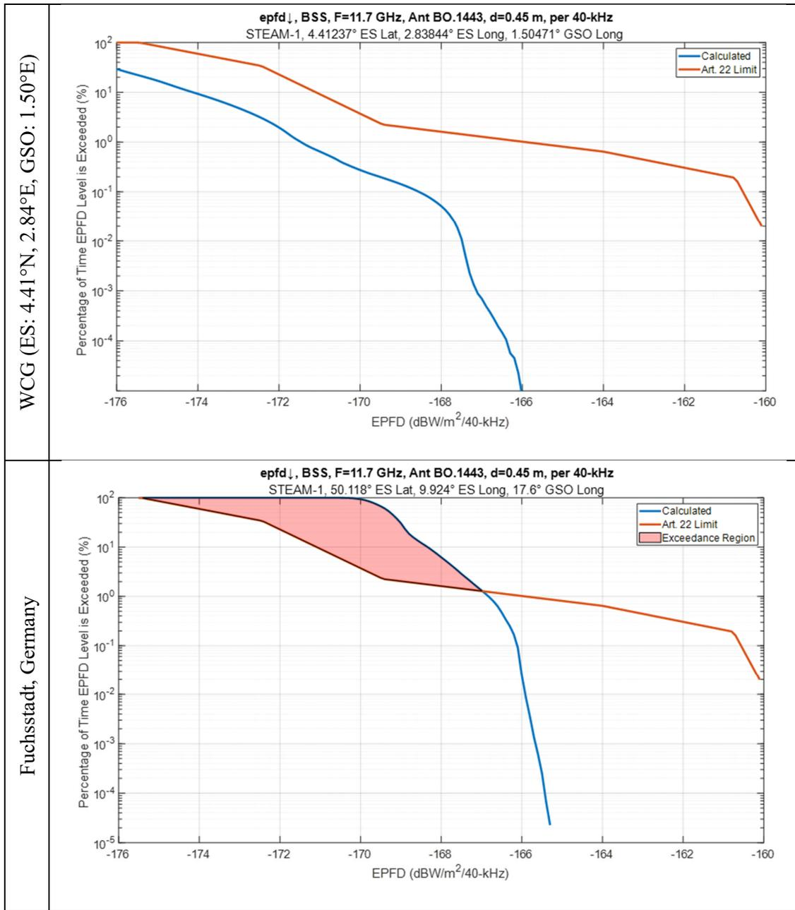
Figure 3 - Comparison of STEAM-1 EPFD ↓ at 11.7 GHz with 0.45 cm GSO ES for WCG and for Fuchsstadt, Germany (50.118°N, 9.924°E) with GSO Satellite at 17.6°E
