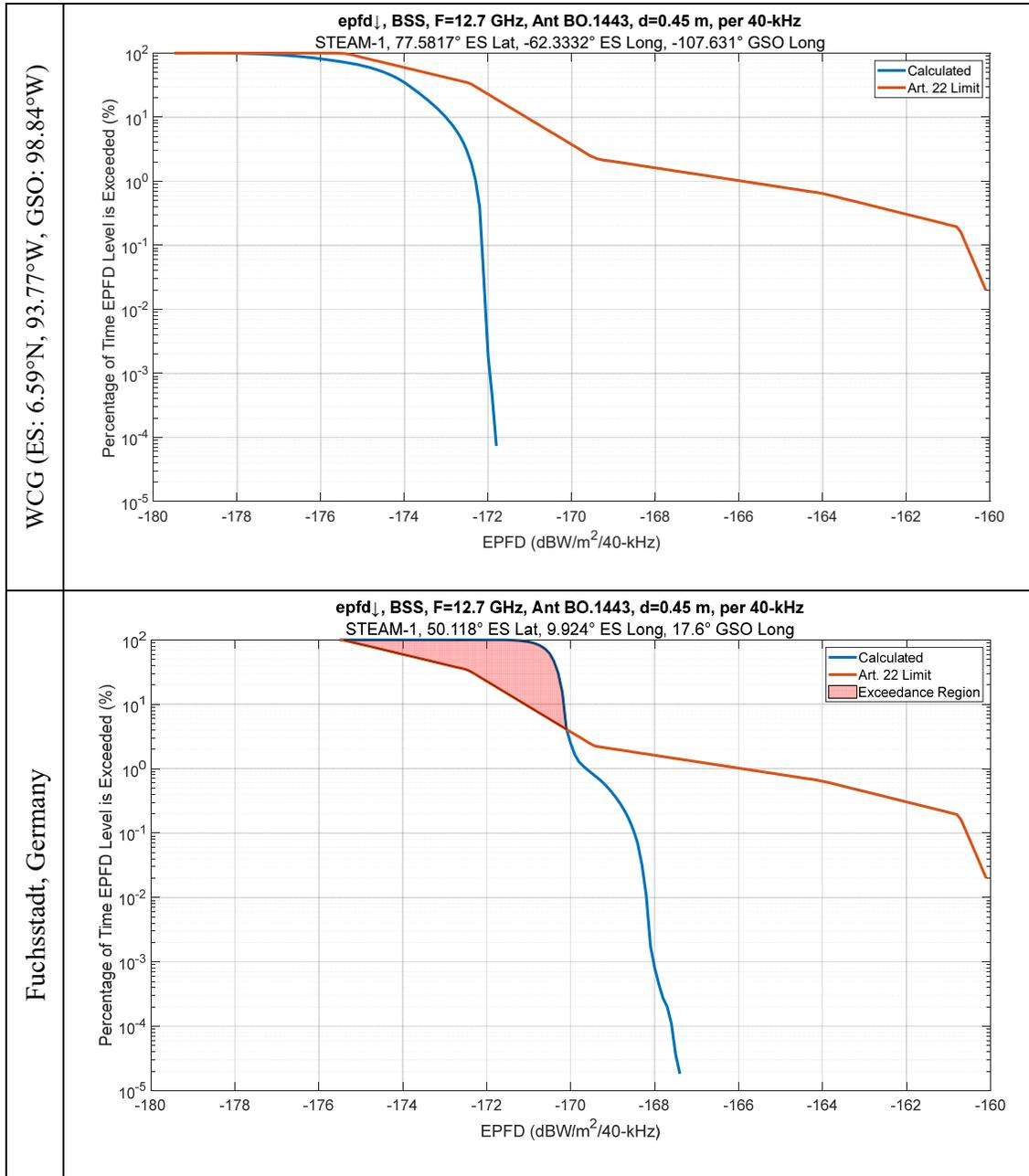
Figure 17 – Comparison of STEAM-1 (ID 121520025) EPFD<sub>↓</sub> at 12.7 GHz with 0.45 m GSO ES for WCG and for Fuchsstadt, Germany (50.118°N, 9.924°E) with GSO Satellite at 17.6°E
