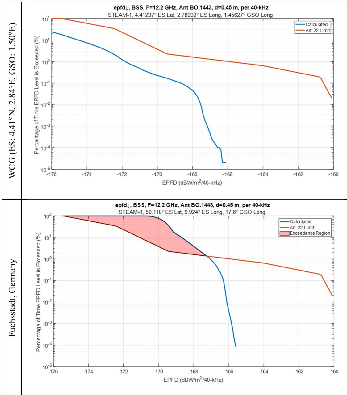
Figure 6 - Comparison of STEAM-1 EPFD<sub>↓</sub> at 12.2 GHz with 0.45 cm GSO ES for WCG and for Fuchsstadt, Germany (50.118°N, 9.924°E) with GSO Satellite at 17.6°E
