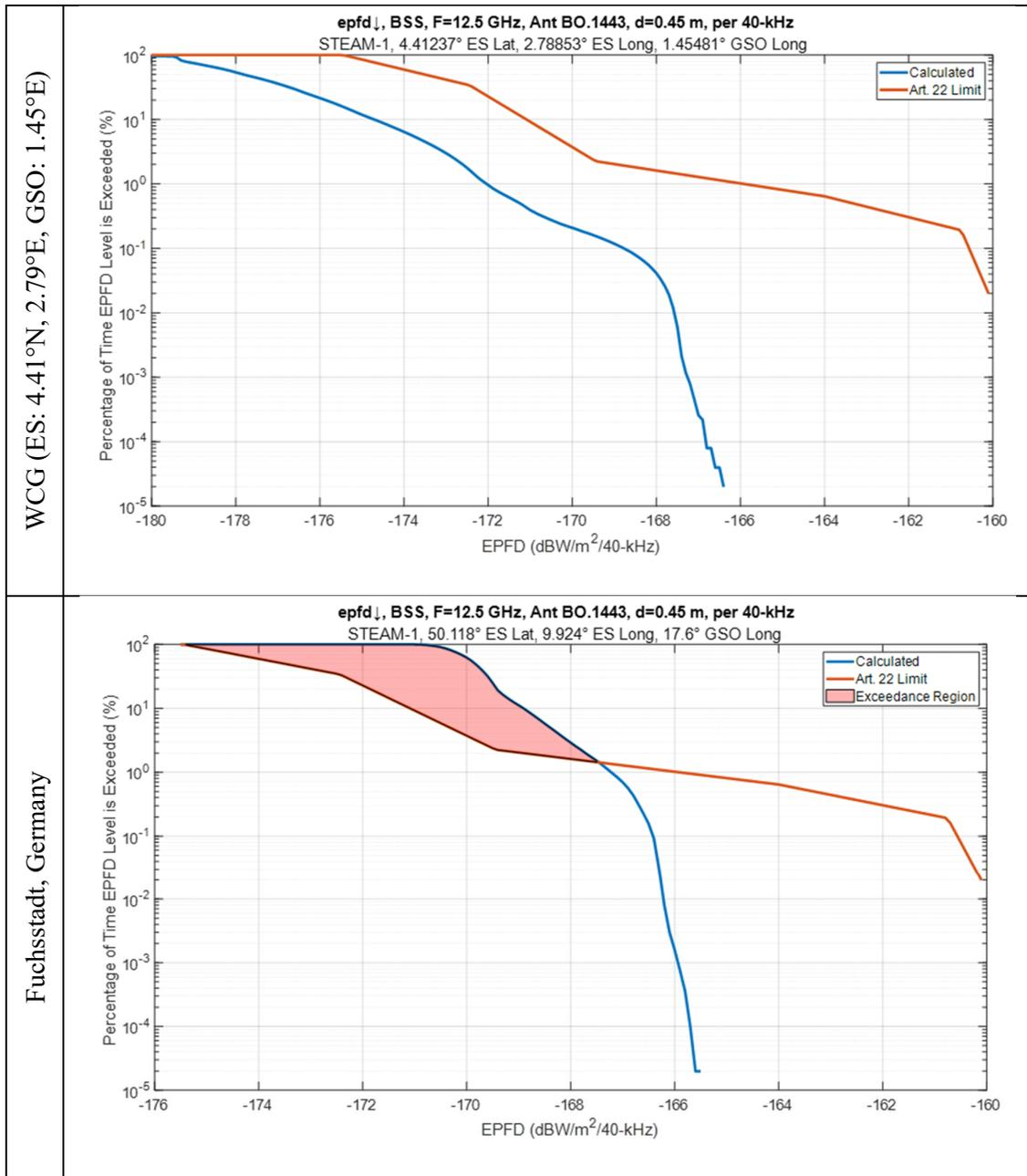
Figure 9 - Comparison of STEAM-1 EPFD↓ at 12.5 GHz with 0.45 GSO ES for WCG and for Fuchsstadt, Germany (50.118°N, 9.924°E) with GSO Satellite at 17.6°E
