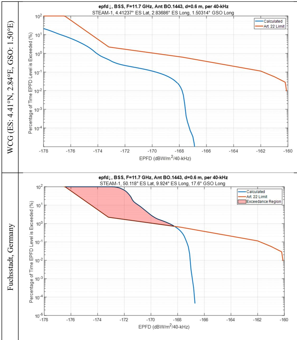
Figure 4 - Comparison of STEAM-1 EPFD ↓ at 11.7 GHz with 0.6 m GSO ES for WCG and for Fuchsstadt, Germany (50.118°N, 9.924°E) with GSO Satellite at 17.6°E
